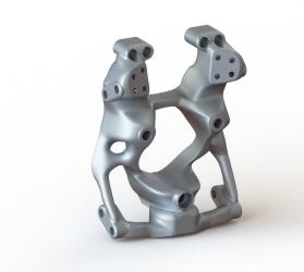
With SOLIDWORKS Simulation Professional topology study capabilities, Giaffone Racing is designing new components for the Brazilian Stock Car series, beginning with the suspension upright, or knuckle, shown here, which attaches the wheel, brake rotor, hub, brake caliper, and steering arm to the vehicle. With a SOLIDWORKS topology study, Giaffone optimized this component to reduce weight while maintaining stiffness.
